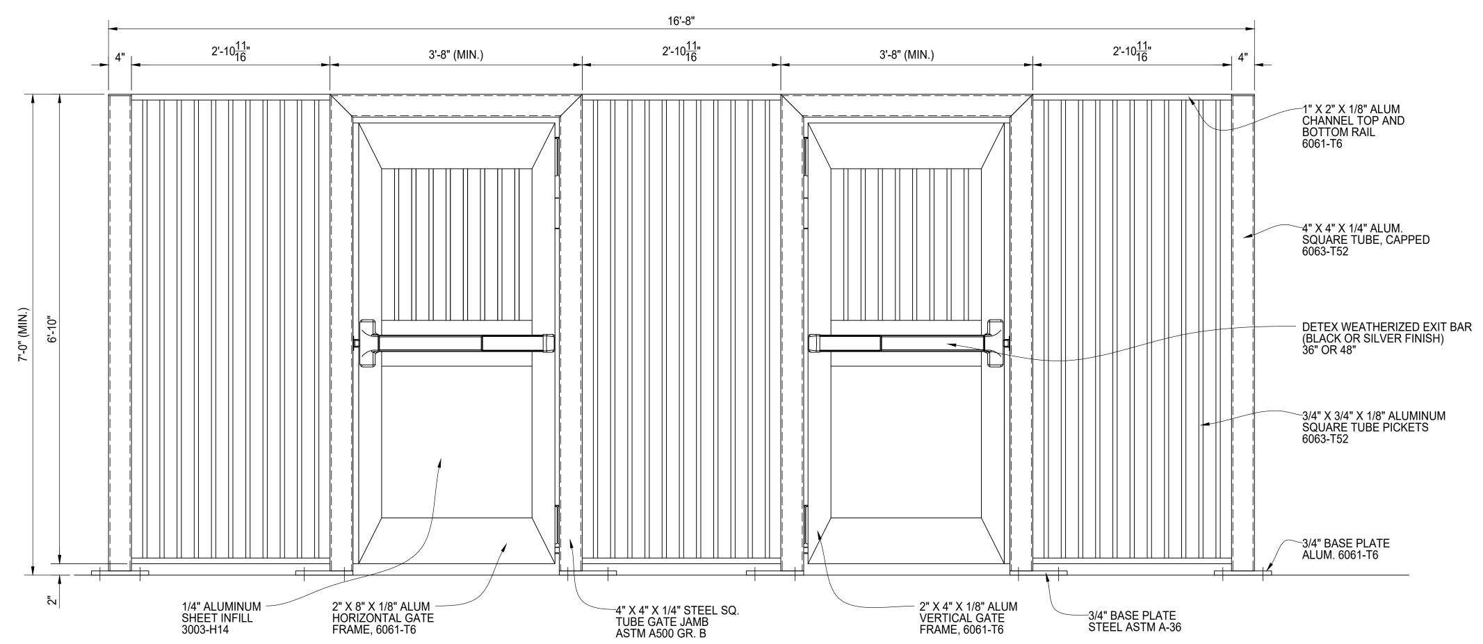
SEE SHEET 06 FOR GATE HARDWARE DETAILS. LATCH HANDLE TO BE 42" ABOVE GRADE.
