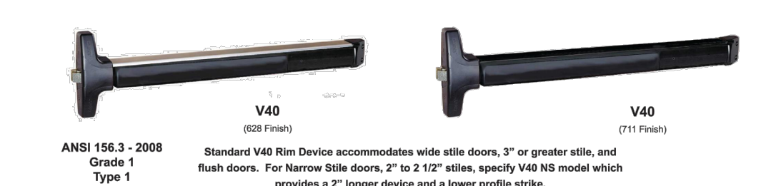
ANSI 156.3 - 2008 Grade 1 Type 1 Standard V40 Rim Device accommodates wide stile doors, 3" or greater stile, and flush doors. For narrow stile doors, 2" to 2 1/2" stile, specify V40 NS model which provides a 2" longer device and a lower profile strike.
