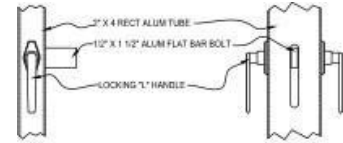
GATE LATCH DETAIL
