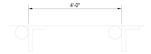
Ordinate dimension are dimensions that are measured from a zero ordinate or benchmark. Ordinate dimensions are usually a better choice for taking field dimension of a run with multiple points. With the dimensions all being pulled from the same zero point, there is less room for error.
