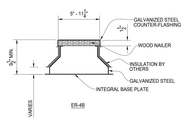
ER-4A/ER-4B - EQUIPMENT RAILS FOR INSULATED DECKS
