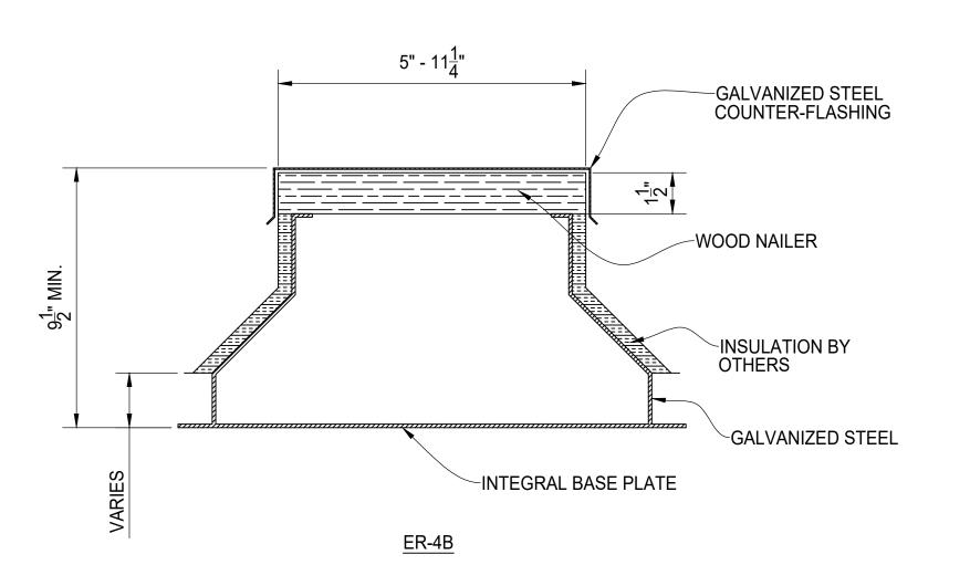
ER-4A/ER-4B - EQUIPMENT RAILS FOR INSULATED DECKS
