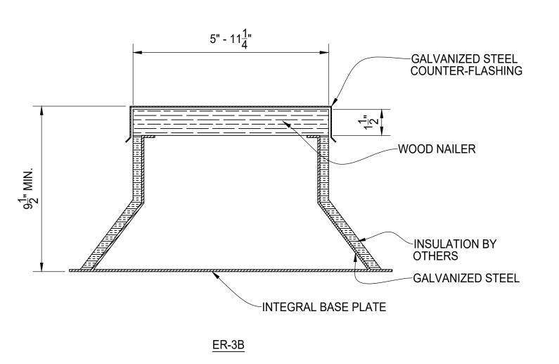
ER-3A/ER-3B - EQUIPMENT RAILS FOR UNINSULATED DECKS
