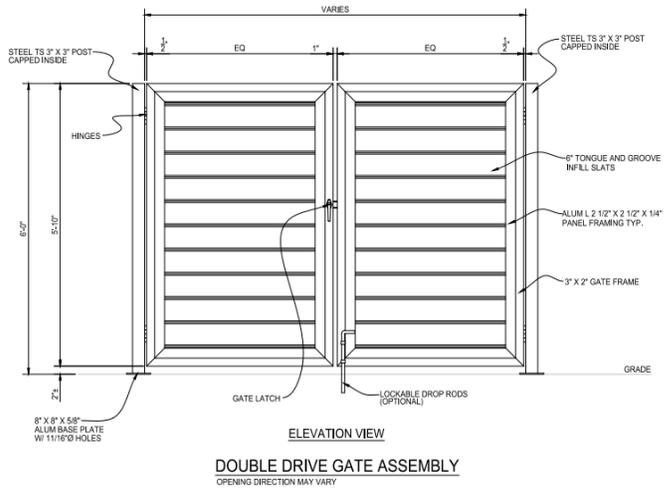
4. Welded frame, size as shown on the contract drawings, extruded aluminum tubing with aluminum fixed panels to match
