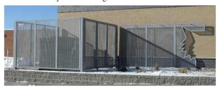
a. Louvers. The most widely used mechanical equipment screening is louvers. Louvers are available in vertical, horizontal and diagonal. Louvers may be spaced such to allow more or less visibility between the louvers and opennes.
