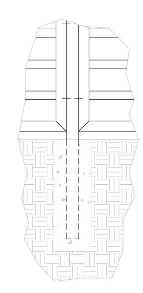
POST CAN BE SET WITH EITHER A BASE PLATE (SHOWN AT LEFT) OR EMBEDDED IN A FOOTING. IF USING A FOOTING, DEPTH AND DIAMETER TO BE DETERMINED BY END USER.
