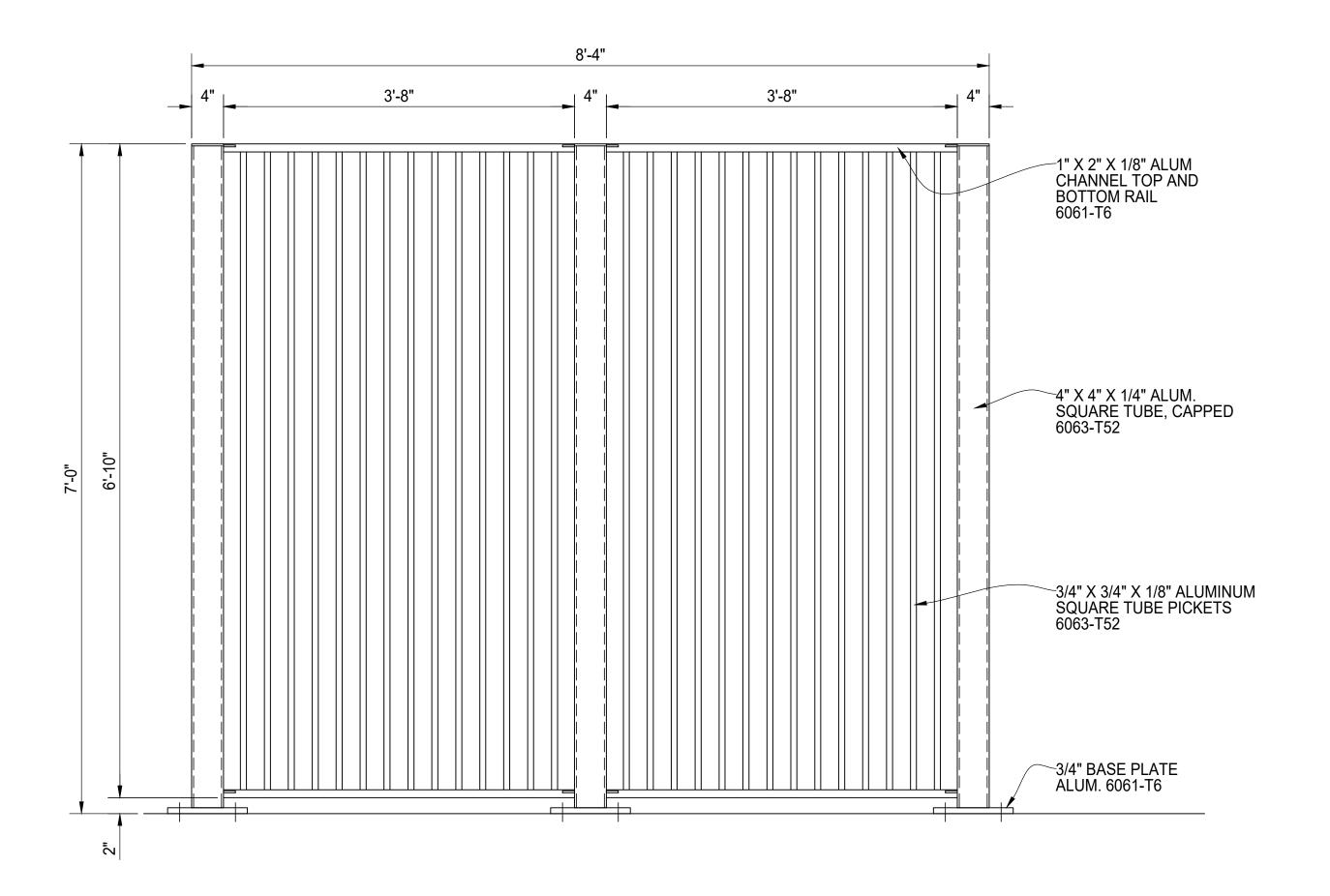
PEDESTRIAN GATE ENTRY - PANEL ELEVATION VIEW
